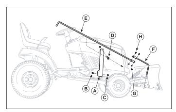
Figure 13. Blade Control Arm Installation
